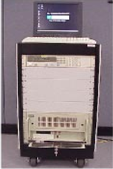
Fig. 4. The transceiver rack front-end for 6 transmit/12 receive antennas.
